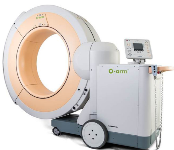
Fig. 8 The O-arm mobile surgical cone beam CT imaging device (Medtronic GmbH, Earl-Bakken-Platz 1,40670 Meerbusch, Germany)
